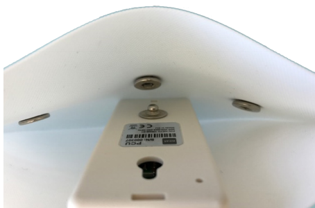
Picture 10. Fasten the main unit to the anchor.
