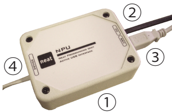
Picture 1. Connectors and cables on the NPU
